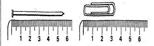
Look at the picture of the nail next to the ruler. The nail is 57 mm long. This is 5 cm + 7 mm. There are 10 mm in each cm, so 1 mm = 0.1 cm (one-tenth of a centimetre). This means that 7 mm = 0.7 cm, so 57 mm = 5 cm + 7 mm
